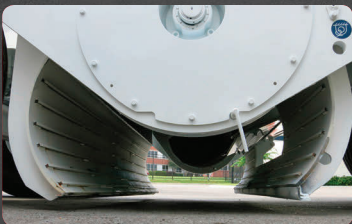
Full width cleanout doors on C1 & C2 give incredible access
