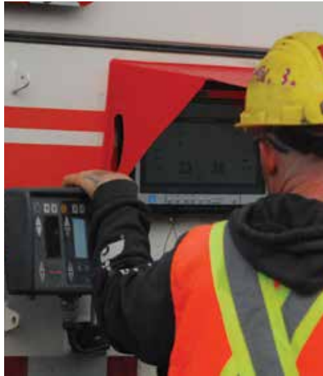
The cutting-edge 3D milling technology allows for variable milling depth on a road, resulting in perfect smoothness.
