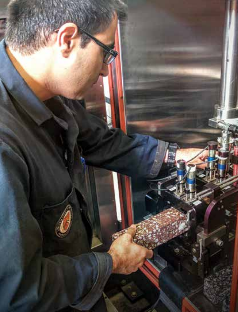
Figure 1. Four-point bending beam setup used in testing long-term durability of asphalt mixtures under repeated cyclic fatigue at certain strain level and climate conditions.
