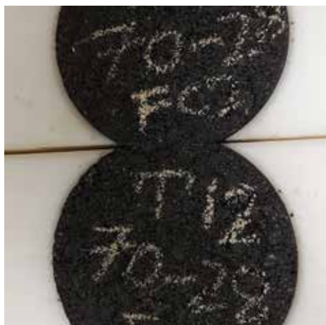
Figure 3. Hamburg Wheel Rut Tester to evaluate the stability of the aggregate skeleton and stiffness of the binder at certain temperatures while the sample is being submerged in hot water, indicating any moisture susceptibility concerns with the aggregate and binder compatibility. Also shown is the before and after of a mix tested by a Hamburg wheel.
