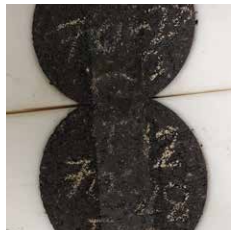
Figure 3. Hamburg Wheel Rut Tester to evaluate the stability of the aggregate skeleton and stiffness of the binder at certain temperatures while the sample is being submerged in hot water, indicating any moisture susceptibility concerns with the aggregate and binder compatibility. Also shown is the before and after of a mix tested by a Hamburg wheel.
