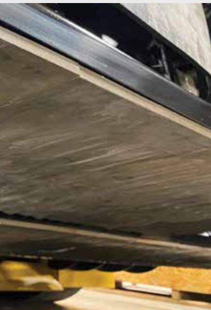
Close view of the surface of the mat after paving with the SDX screed. (Caterpillar)
